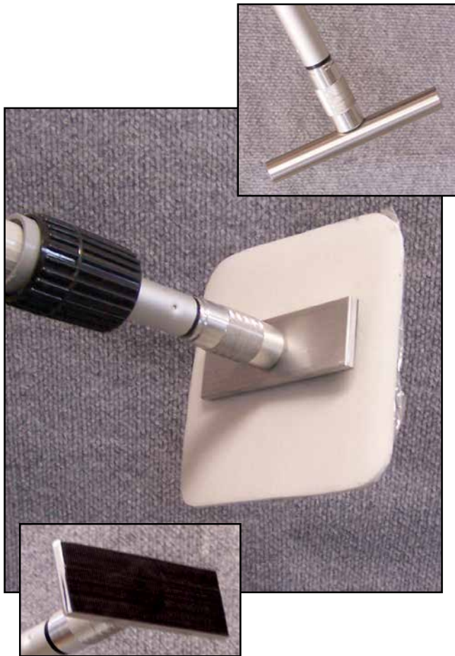
The Trenton Keyhole Patch-Pad applicator tool has a velcro surface (left) for holding the Patch-Pad. The center picture shows the applicator tool with an attached Patch-Pad that has pre-applied coating. The finishing tool (right) is used to press the Patch-Pad onto the pipe.
